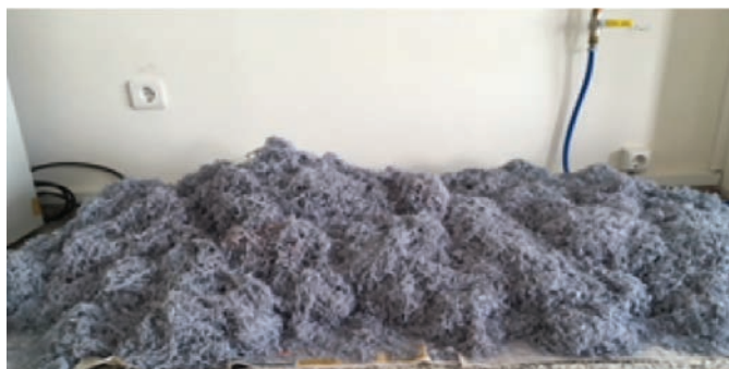
Figure 1. Shaving wastes containing chromium
