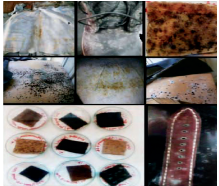
Figure 2. Fungal infested leather samples collected from various tanneries
