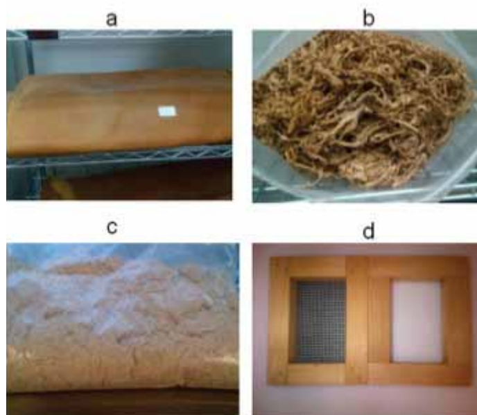
Figure 1. Vegtan split (a), strips of vegtan split (b), fibers after Wiley Mill grinding (c), and paper making kit (d).
