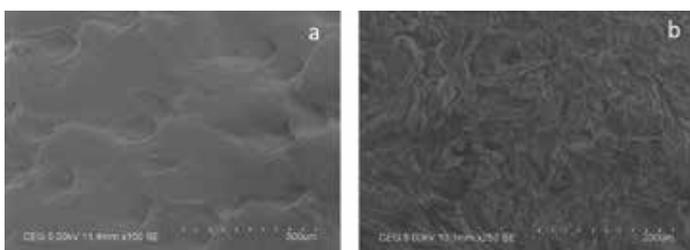
Figure 4. Scanning electron micrographs of (a) grain and (b) cross section of crust leathers rechromed with SYN1.
