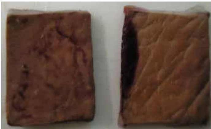
Figure 8. Stain on the vegetable-tanned leather samples caused by Penicillium herguei .
