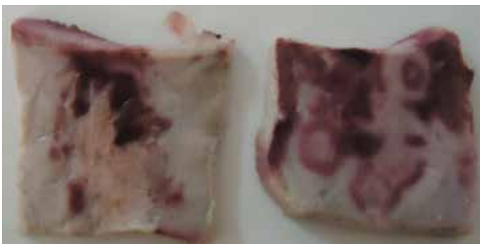
Figure 3. Stains and degradation of pickled hide samples degraded by Penicillium herguei .
