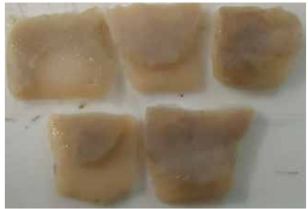
Figure 4. Degradation of pickled hide samples caused by Aspergillus niger .
