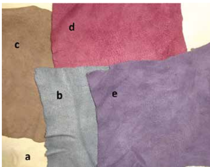
Figure 4. Photograph of a) un-dyed chamois, chamois leather with dye (2%) b) Tancol Black LSG c) Tancol Chocolate Brown LFP d) Tancol Brown LSG and e) Tancol Prune LBRS.
