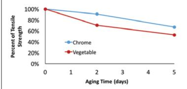
Figure 10. Averages of tensile strength retention (tensile strength after aging/tensile strength at time=0) for all samples tested in a manner that replicates Piltingsrud's experiment.<sup>2</sup>
