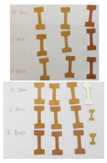
Figure 3. Pictures of the seven different vegetable tanned samples after aging prior to being tested in the tensile apparatus.
