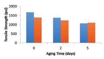
Figure 9. Tensile strengths of individual chrome tanned leathers. The colors and order of the bars refer to the same leather.
