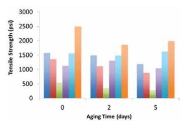
Figure 7. Tensile strengths of individual vegetable tanned leathers. The colors and order of the bars refer to the same leather. Specifically, starting from the left, all of the dark blues at 0, 2 and 5 days correspond to the same leather, while the reds correspond to the same leather etc.
