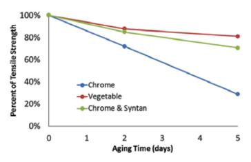
Figure 5. Averages of tensile strength retention (tensile strength after aging/tensile strength at time=0) for all samples tested at the three different times after aging started (time=0 corresponds to unaged samples). If a sample could not be tested, then the value was set to 0%.
