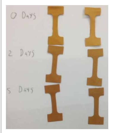
Figure 4. Pictures of the two different vegetable tanned samples after aging prior to being tested in the tensile apparatus.
