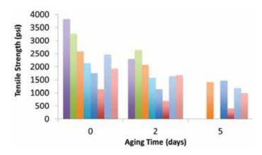
Figure 8. Tensile strengths of individual chrome tanned leathers. The colors and order of the bars refer to the same leather. Missing entries in day 5 are samples that could not be tested because the samples could not be loaded into the tensile machine without breaking.
