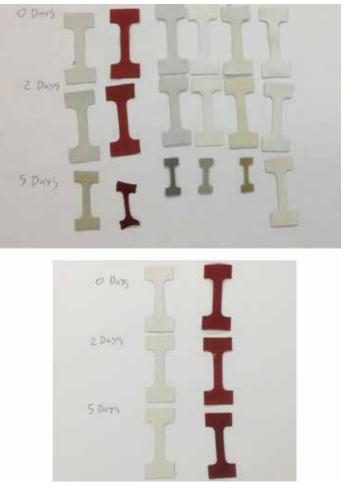
Figure 2. Pictures of the eight different chrome tanned samples after aging prior to being tested in the tensile apparatus. The 5 day samples that are boxed could not be tested.
