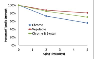
Figure 6. Averages of tensile strength retention (tensile strength after aging/tensile strength at time=0) for samples tested at the three different times after aging started (time=0 corresponds to unaged samples). If a sample could not be tested, this sample was not included in the average (which was the case for three chrome samples.
