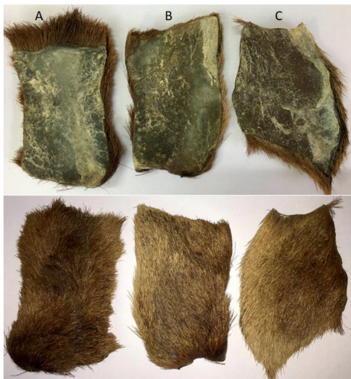
Fig. 2: Photographs of grain and flesh sides of preserved skin samples after 30 days storage at ambient conditions. a. CO 2 , b. CO 2 + acetone, c. wet-salted
