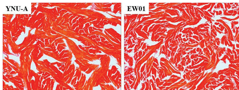
Figure 5. Staining results of collagen fiber in wet blue treated by acidic (YNU-A) or neutral (EW01) protease (100× whole ver. sec.)
