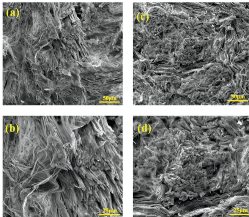
**Figure 5.** SEM micrographs of the cross-section of vegetable-tanned leather limed in (a, b) 2% Ca(OH)<sub>2</sub> and (c, d) 7% urea/2% Ca(OH)<sub>2</sub> solutions.
