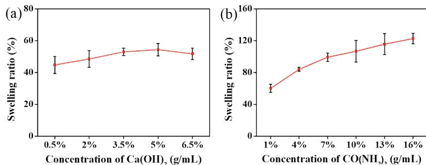
**Figure 3.** Variation of swelling ratio of hides with concentrations of (a)  $\text{Ca}(\text{OH})_2$  and (b) urea (in the presence of 2%  $\text{Ca}(\text{OH})_2$ ).
