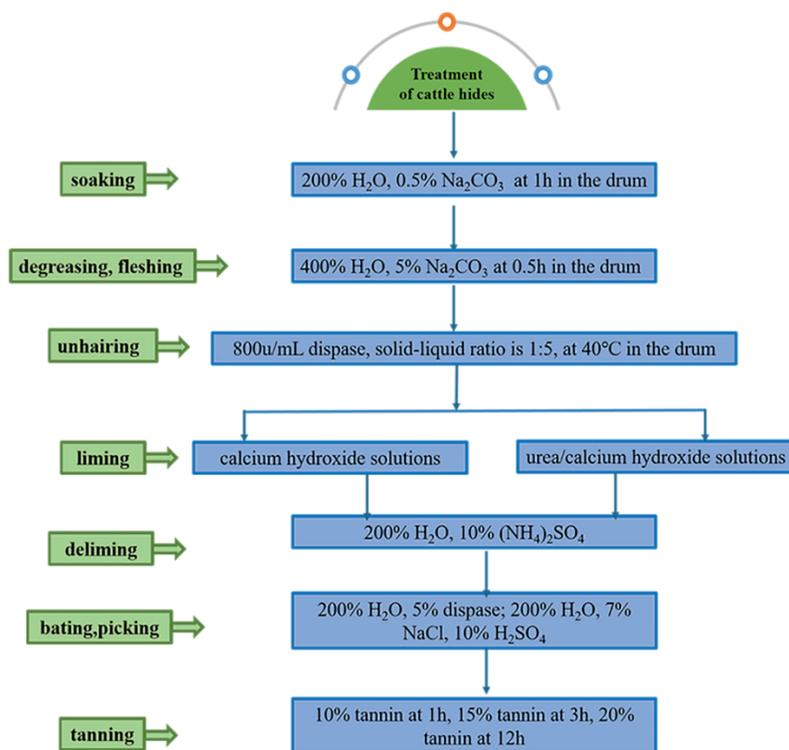
Figure 1. Schematic representation of the overall treatment of cattle hides.
