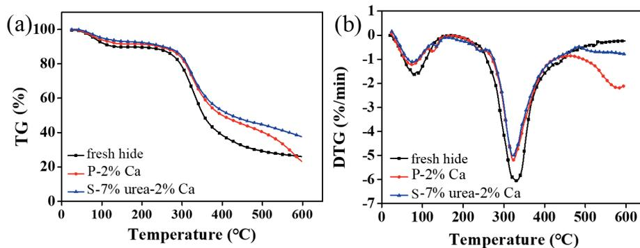
Figure 6. (a) TG and (b) DTG curves of hides limed by different liming systems.
