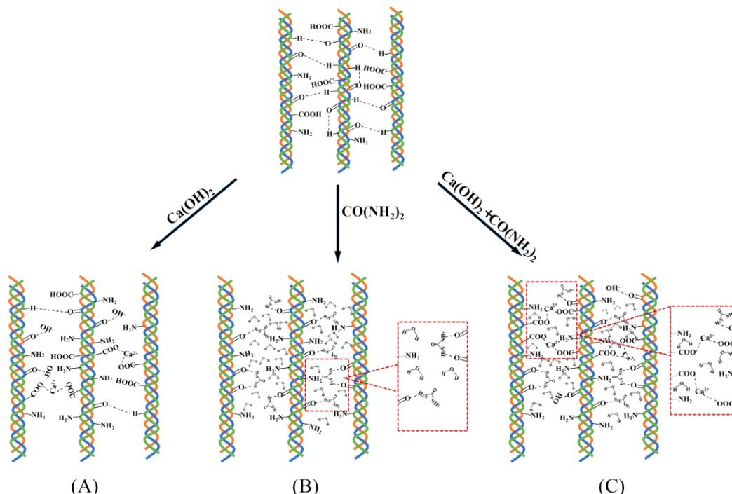
Figure 7. The mechanism of liming in (A) calcium hydroxide and (C) urea/calcium hydroxide solution; (B) The disrupting mechanism of hydrogen bonding in collagen matrix by urea.
