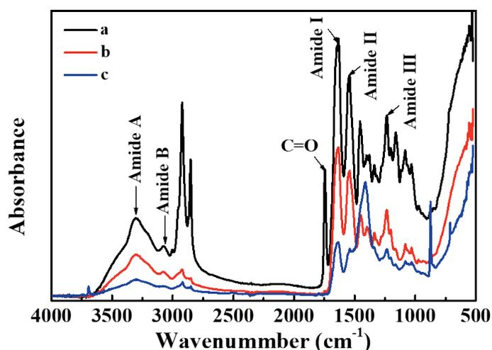
Figure 8. FTIR spectra of (a) fresh hide, (b) P-2%Ca, (c) S-7%urea-2%Ca.
