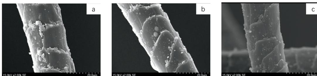
**Figure 7.** SEM micrographs of wool fibers under different pressures (a, b and c represent wool fibers before treatment, after 0.2 MPa subcritical n-pentane and 0.6 MPa subcritical n-pentane).
