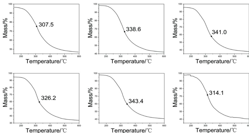
Figure 3. TG analysis curves of wool fibers under different pressures (a, b, c, d, e and f is blank sample, 0.2Mpa, 0.3Mpa, 0.4Mpa, 0.5Mpa and 0.6Mpa).
