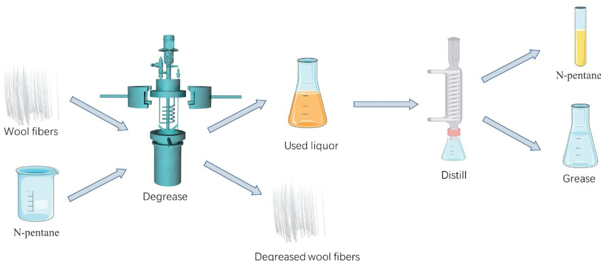
Figure 1. The wool fibers degreasing procedure with subcritical n-pentane.
