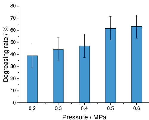
Figure 2. Degreasing rate at different pressures.
