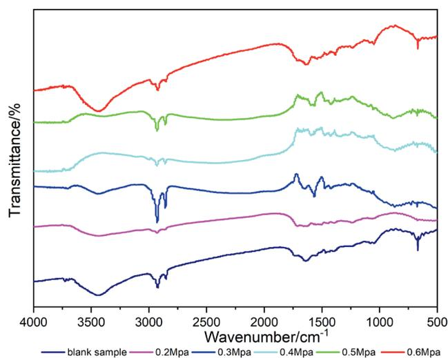
Figure 4. FT-IR analysis of wool fibers at different pressure.
