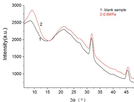
Figure 6. X-ray powder diffraction analysis of wool fibers under different conditions.
