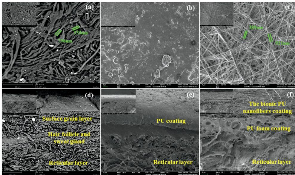
**Figure 2.** (a) SEM of the surface of FGL. (b) SEM of the surface of PUSL. (c) SEM of the surface of NBSL. (d) SEM of longitudinal section of FGL. (e) SEM of longitudinal section of PUSL. (f) SEM of longitudinal section of t NBSL.
