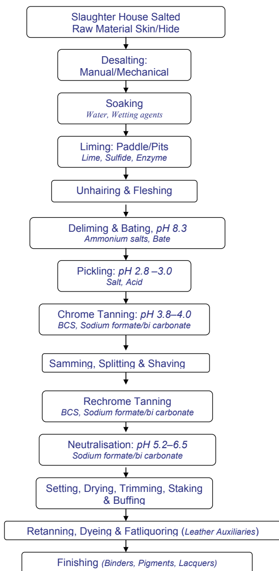
Figure 2. Flow chart for chrome tanning process
