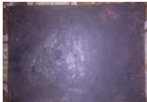
Figure 3. Melting Shredded HDPE waste plastic using metal pot by electrical stove and molded cutting board
