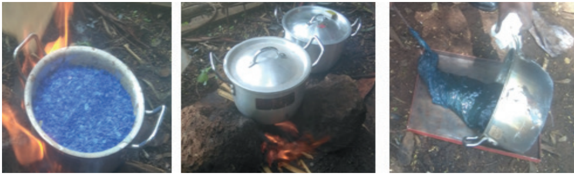
Figure 4. Melting Shredded HDPE waste plastic using metal pot by wood fire and plastic, and molded cutting board
