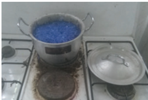
Figure 3. Melting Shredded HDPE waste plastic using metal pot by electrical stove and molded cutting board
