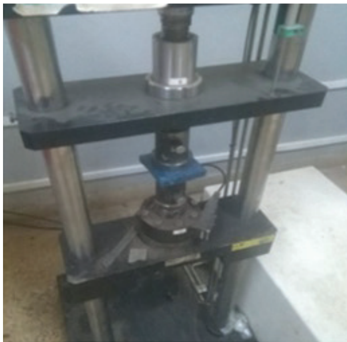
Figure 10. Developed cutting board compression test.
