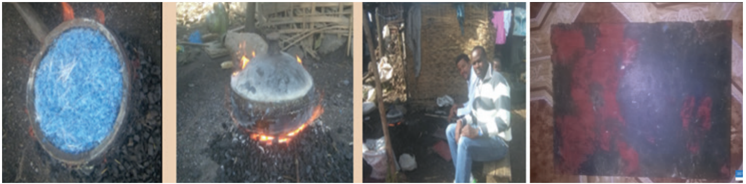
Figure 6. Melting Shredded HDPE waste plastic using clay pot by charcoal stove with fire blowing fan, molded cutting board
