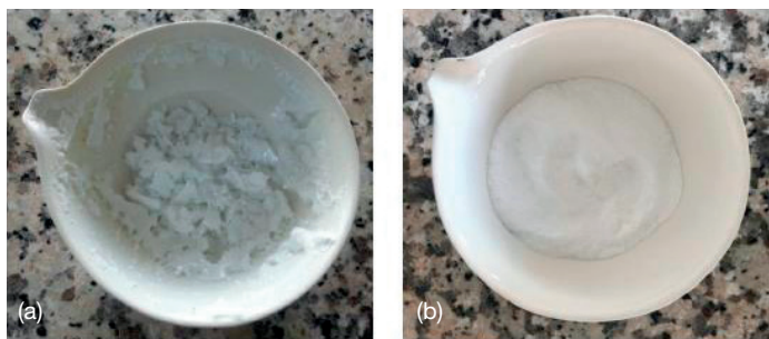
Figure 1. Oxidized starch: after dry in oven (a) and after grind (b)
