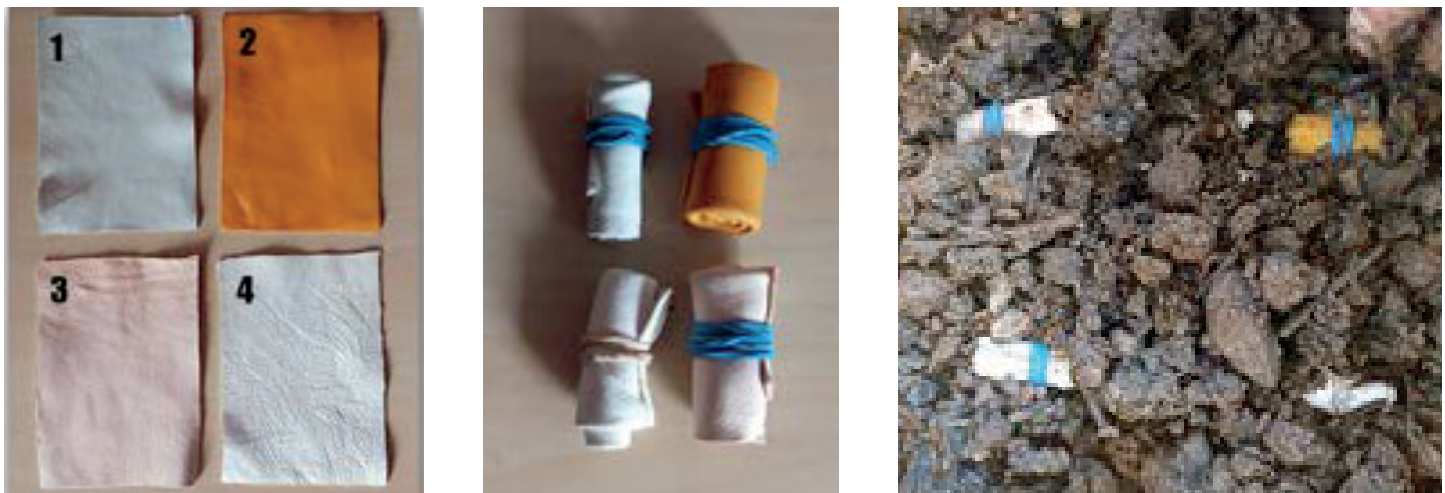
Figure 1. Natural biodegradation test for sheep skin
