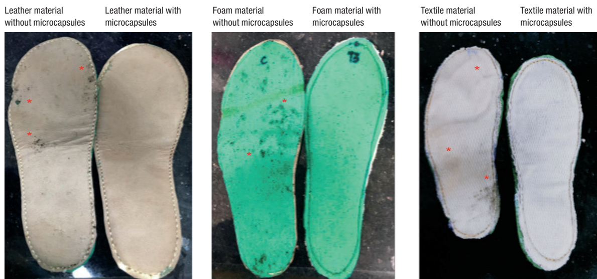
Figure 4. Antifungal activity of a complete foot-bed materials fused with mixed herbal oil microcapsules in comparison with the materials without microcapsules. The images were taken after day 7 of the experimental period.
