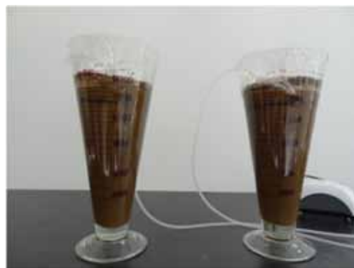
Figure 1. Aeration device for biological wastewater treatment
