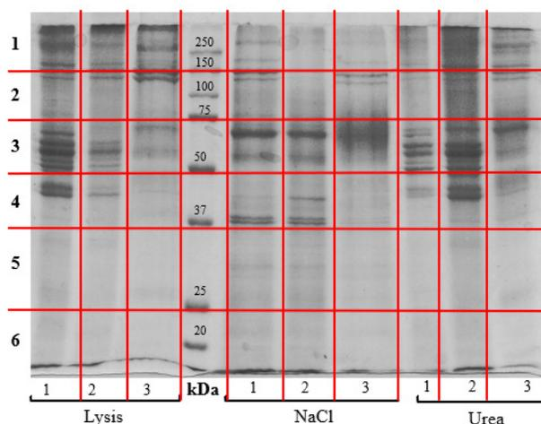
**Figure S3.** Diagram of how the SDS-PAGE gels were manually cut.
