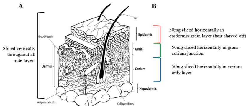
**Figure S2.** Diagram of how the hide was sliced (A) for confocal microscopy images (60µM thick slices) and (B) for protein extraction (10µM thick slices).
