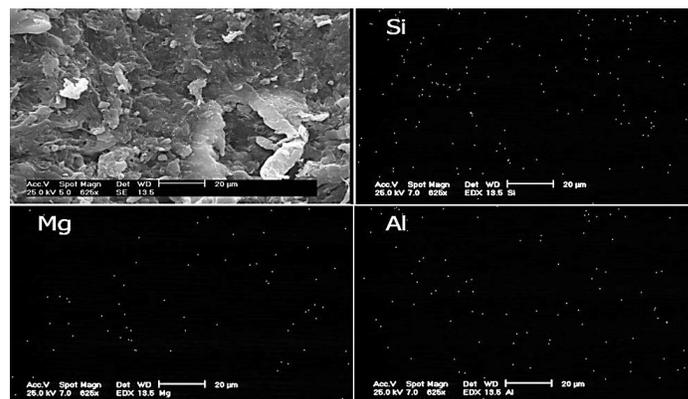
**Figure 5.** Elemental analysis of sample: leather-Na<sup>+</sup>Mt\_5%.
