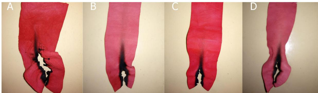
**Figure 10.** Goat samples evaluated by flammability vertical test according to 14 C.F.R. Appendix F to Part 25 Part I (a) (1) (i). (A) leather, (B) leather- Na+Mt\_1%, (C) leather- Na+Mt\_3% and (D) leather- Na+Mt\_5%.
