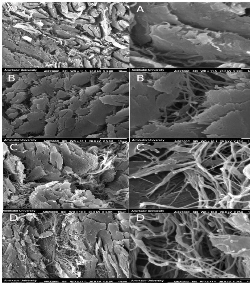
**Figure 7.** Cross sectional SEM images of bovine leather at 500 and 2000X magnification, respectively; (A) leather, (B) leather-Na<sup>+</sup>Mt\_1%, (C) leather-Na<sup>+</sup>Mt\_3% and (D) leather-Na<sup>+</sup>Mt\_5%.
