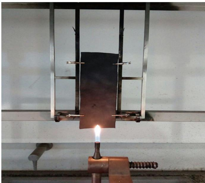
Figure 1. Sample placement for vertical flammability test.
