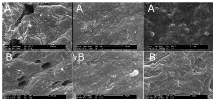
**Figure 3.** Grain surface SEM images of goat leather at 100, 1250 and 20000× magnification, respectively; (A) leather and (B) leather-Na<sup>+</sup>Mt\_3%.
