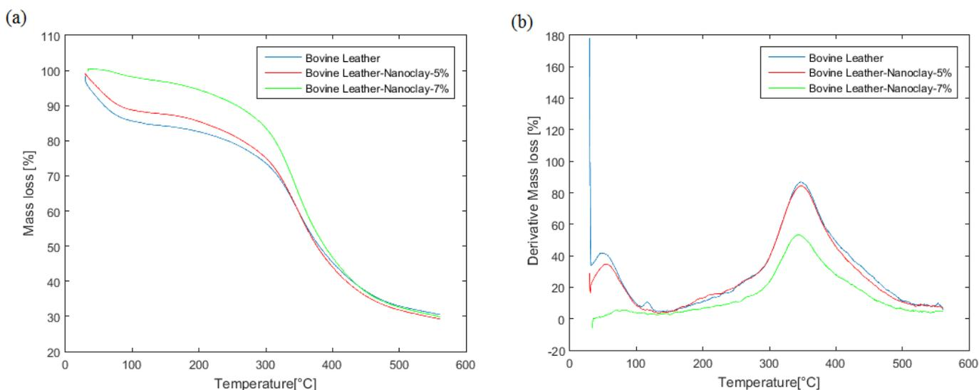
**Figure 2.** (a) TGA and (b) DTG curves of leather samples having different clay content in nitrogen.
