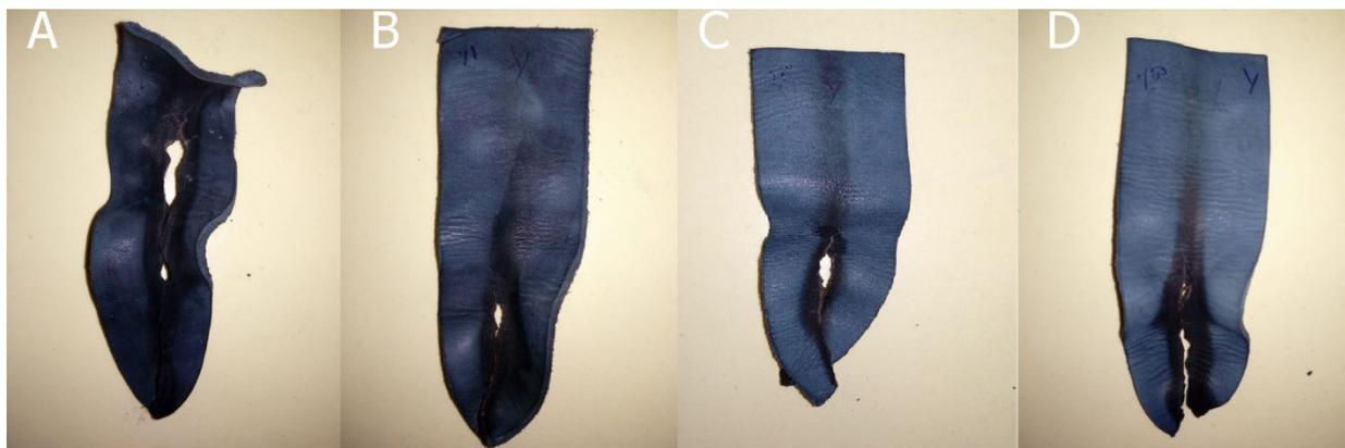
**Figure 9.** Bovine samples evaluated by flammability vertical test according to 14 C.F.R. Appendix F to Part 25 Part I (a) (1) (i). (A) leather, (B) leather- Na+Mt\_1%, (C) leather- Na+Mt\_3% and (D) leather- Na+Mt\_5%.
