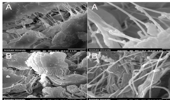
**Figure 6.** Cross sectional SEM images of goat leather at 500 and 2000× magnification, respectively; (A) leather (B) leather-Na<sup>+</sup>Mt\_3%.
