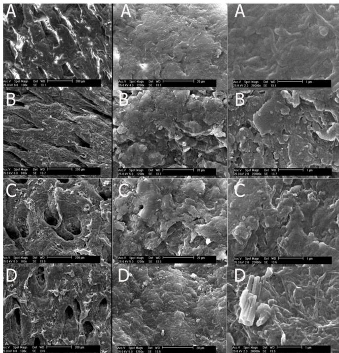
**Figure 4.** Grain surface SEM images of bovine leather at 100, 1250 and 20000× magnification, respectively; (A) leather, (B) leather-Na<sup>+</sup>Mt\_1%, (C) leather-Na<sup>+</sup>Mt\_3% and (D) leather-Na<sup>+</sup>Mt\_5%.
