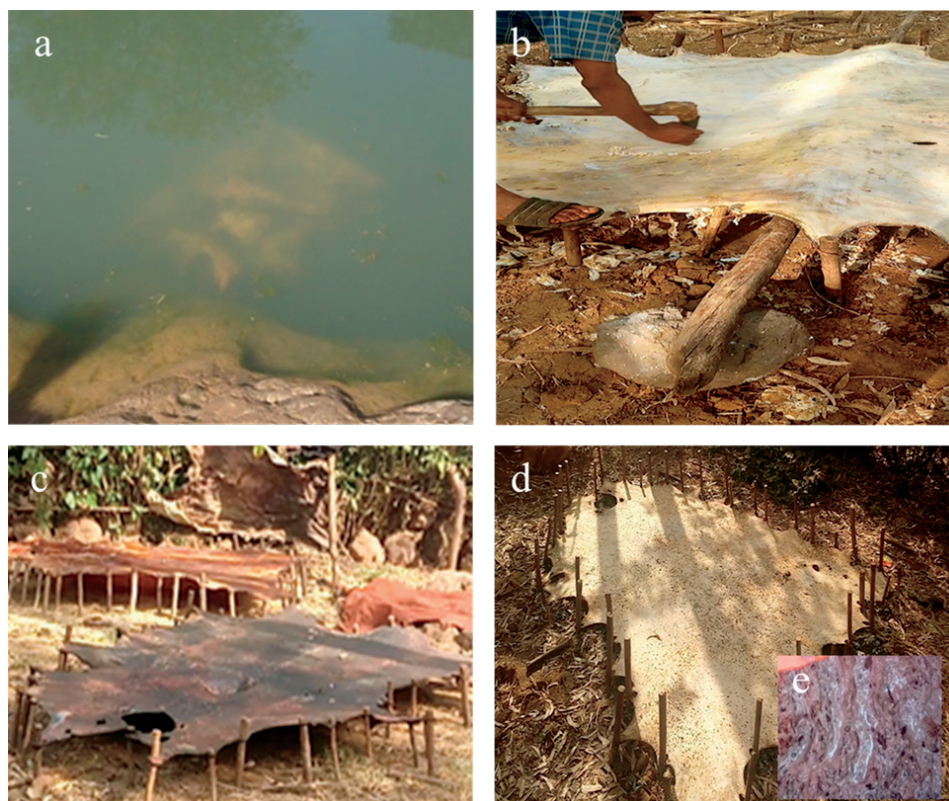
Figure 1. Traditional leather processing in Ethiopia. (a) Hide soaking in damped river, (b) fleshing, (c) cow hides preparation for unhairing, (d) oiling and inset (e) oil used for softening leather.
