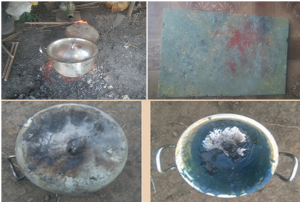
Figure 5. Melting Shredded HDPE waste plastic using metal pot by charcoal stove with fire blowing fan, molded cutting board and failed pot
