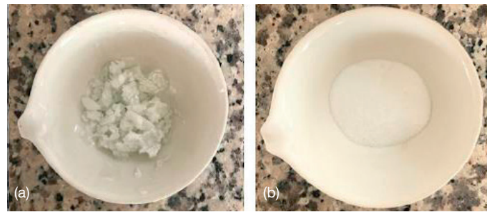
Figure 2. Carboxymethylated starch: after dry in oven (a) and after grind (b)
