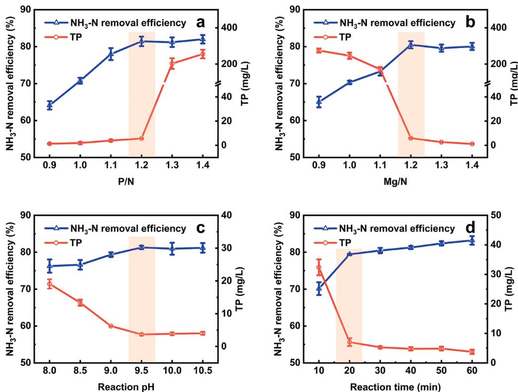
**Figure 1.** Effects of P/N (a), Mg/N (b), reaction pH (c), and reaction time (d) on the removal of  $\text{NH}_3\text{-N}$  from deliming effluent and residual concentration of TP in treated deliming effluent by using MAP precipitation method
