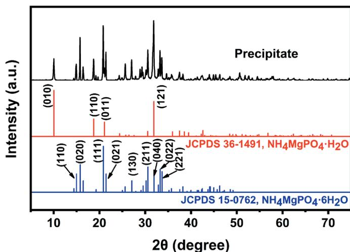
Figure 2. XRD pattern of the precipitate obtained from MAP precipitation treatment of deliming effluent
