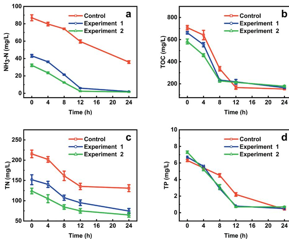
Figure 4. Effect of MAP precipitation method of deliming and bating effluents on aerobic biological treatment of simulated tannery wastewater: (a)  $\text{NH}_3\text{-N}$  concentration; (b) TOC concentration; (c) TN concentration; and (d) TP concentration. Upon the addition of activated sludge, the initial  $\text{NH}_3\text{-N}$ , TOC, TN, and TP concentrations of simulated tannery wastewaters were slightly lower than the values shown in Table 3.
