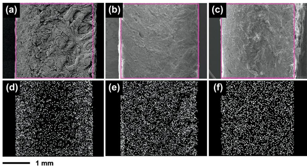
**Figure 4.** SEM images of cross section of Lac-Zr (a), HOS-Zr (b), and chrome (c) tanned leathers. EDS images of the distribution of zirconium/chromium in cross section of Lac-Zr (d), HOS-Zr (e), and chrome (f) tanned leathers.
