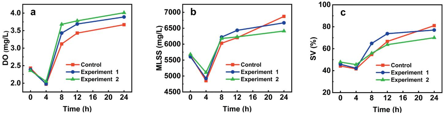
Figure 3. DO (a), MLSS (b) and SV (c) of activated sludge during aerobic biological treatment
