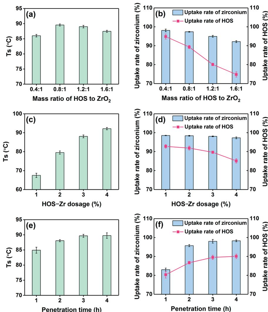
**Figure 1.** Effects of mass ratio of HOS to  $ZrO_2$  (a, b) (HOS–Zr dosage 3%, penetration time 3 h), HOS–Zr dosage (c, d) (mass ratio of HOS to  $ZrO_2$  0.8:1, penetration time 3 h), penetration time (e, f) (mass ratio of HOS to  $ZrO_2$  0.8:1, HOS–Zr dosage 3%) on  $T_s$  of wet white and uptake rate of zirconium and HOS by leather.
