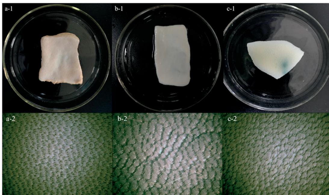
**Figure 6. 1:** Unhairing performance on goatskins by different unhairing methods.
