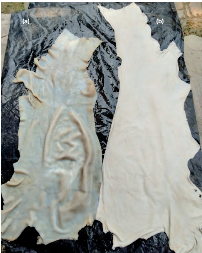
Figure 1. Photographic image of (a) acid swollen pelt and (b) conventional pickled pelt
