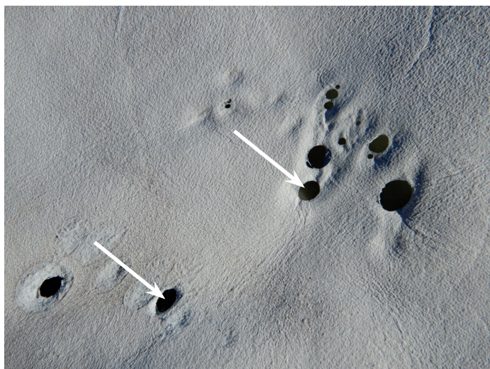
Figure 8. Holes due to bacterial degradation
