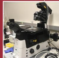
Figure 2. Nikon Eclipse Ti2 microscope (left) used to capture and analyze images. Reactor (right) with plastic tube and glass cover slip with air hose and filter to pump in gas (oxygen or nitrogen).
