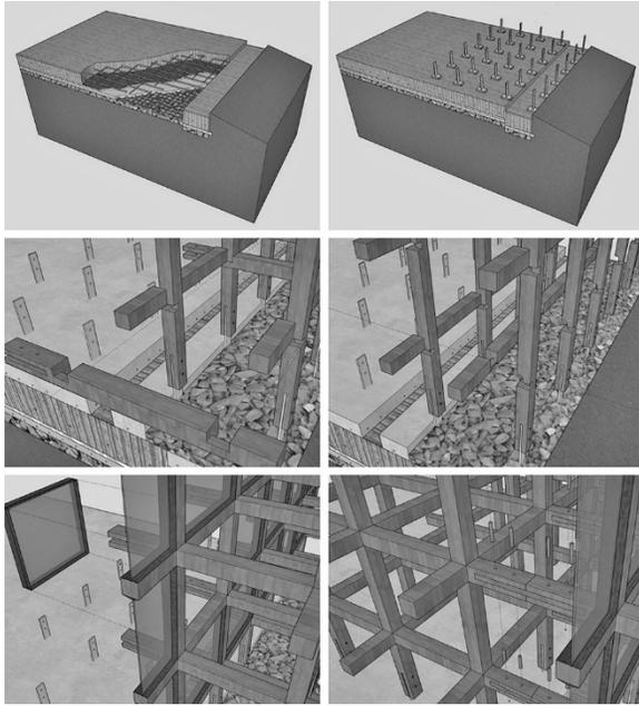
Figure 4 (left): Partial Storyboard Sequence – GC Prostho Museum and Research Center, Kengo Kuma – Drawing by ARCH242 S17 Group 10 (T. Hefler, B. Bangert, R. Taylor) (text removed for clarity)
