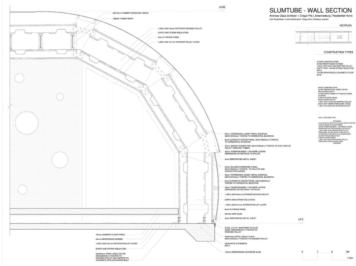
Figure 7: Wall Section – Slumtube, Schnetzer and Pils – Drawing by ARC242 S17 Group 3 (E. Leandro, L. McClanahan, D. Ortiz, K. Rowbotham)
