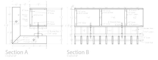
Figure 8: Section Drawings – Detail of Sirch Woodworking by Baumslager and Eberle – Drawings by ARC242 S17 Group 12 (C. Overmyer, R. Hoppe, and A. Bailey)
