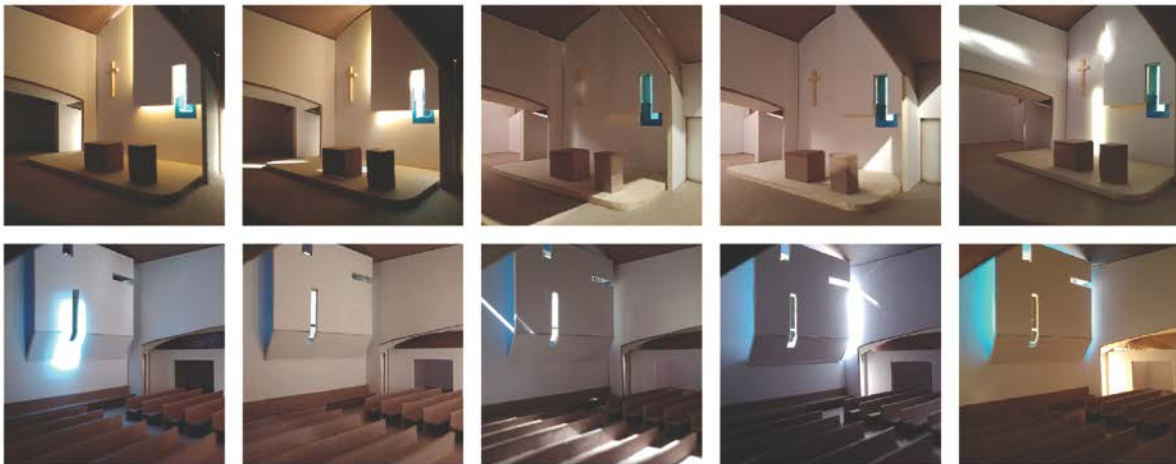
Figure 5 interior of model showing how light changes over the course of the day by anderson yauripoma
