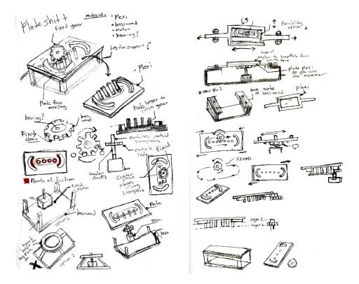
Figure 2. Studies of simple and recognizable mechanisms with a single motion. These early conceptual sketches show an understanding of key features including physical controls and constructions.
