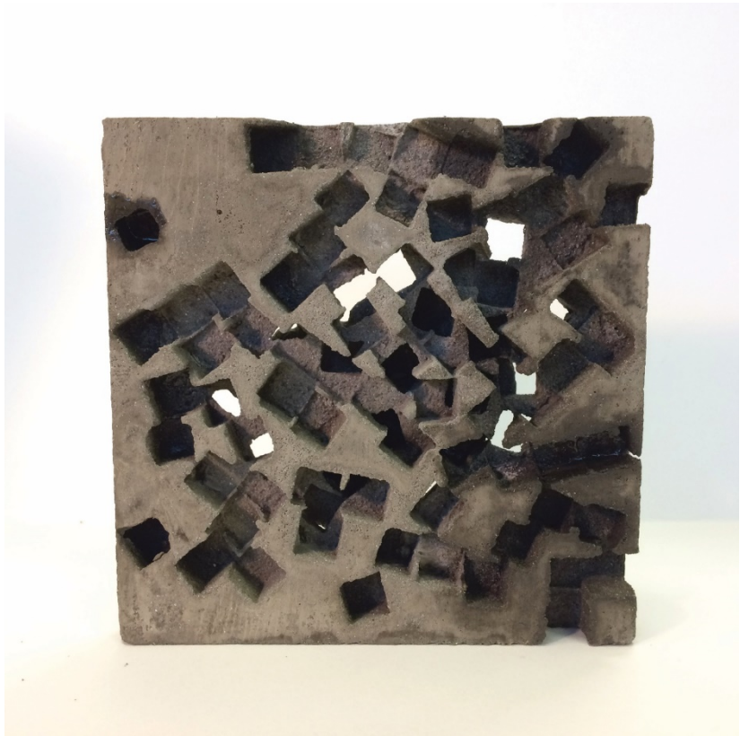
Fig. 7. Cast concrete construction units with variation caused by sugar aggregate that dissolved slowly throughout the curing process (credit: student B. Cunningham)
