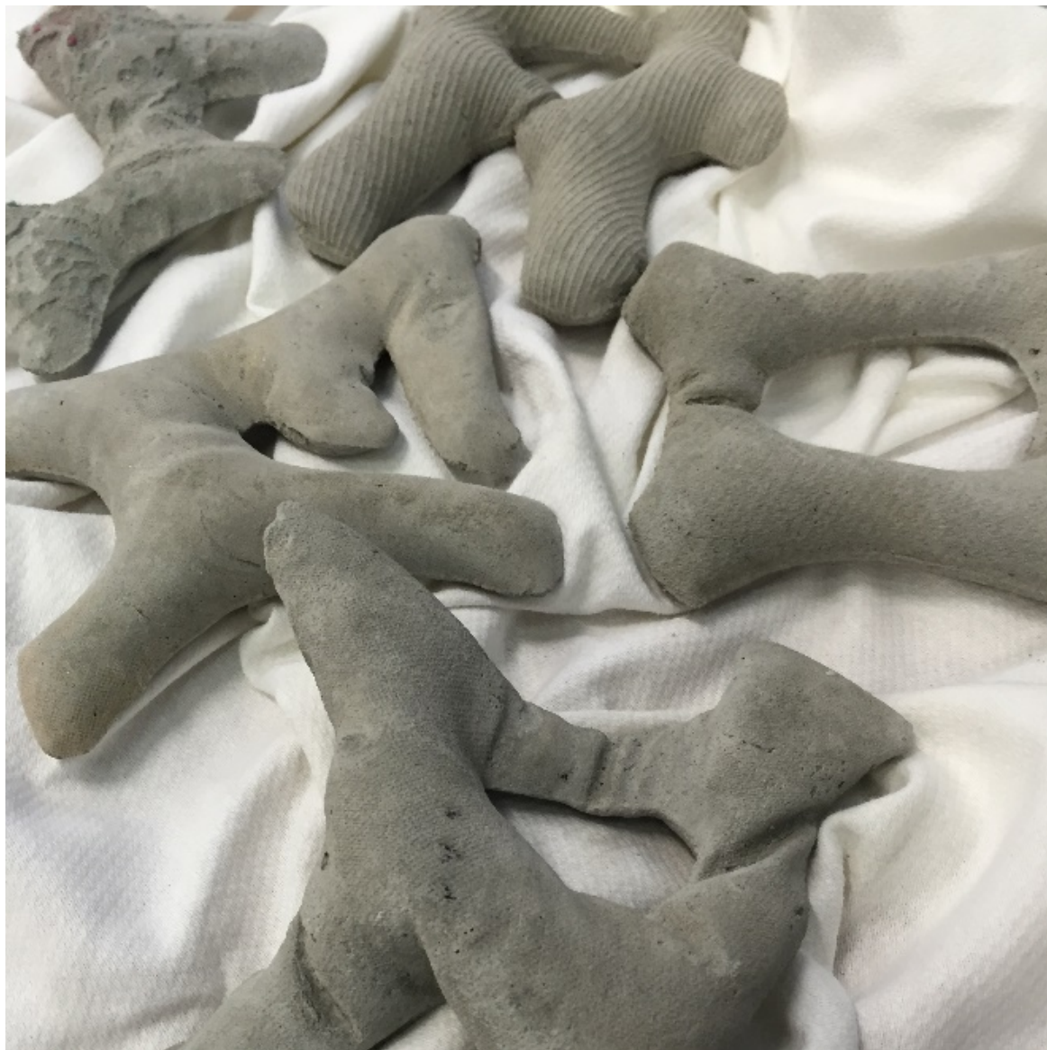
Fig. 3. Cast concrete construction units with variation caused by the use of fabric formwork (credit: student A. Hickerson)
