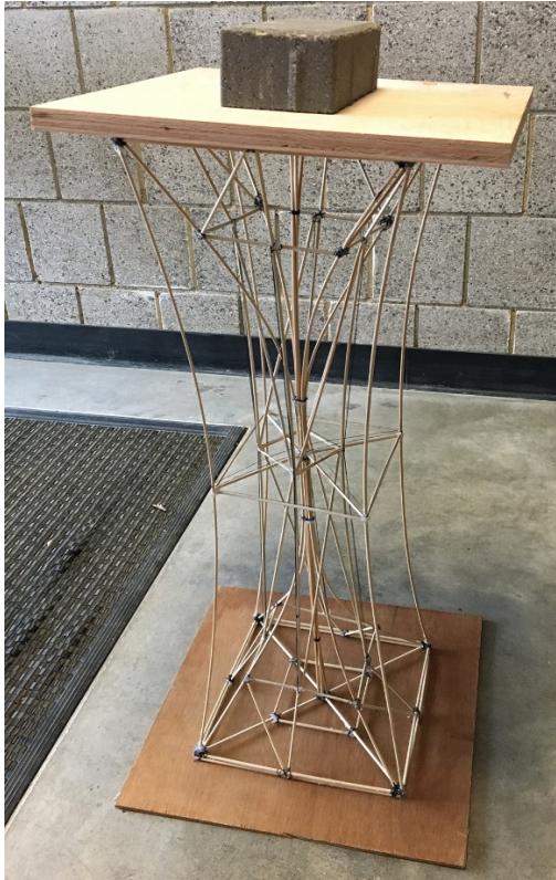
Figure 3: Testing of hollow column/stick tower to meet minimum required loading and consideration of transfer of loads between members and behavior of assembly. Student design by Jake Kriech, Adam Freeby, and Nicholas Bloom. Photo by author.
