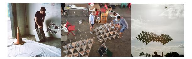
Figure 8, 9, 10. Cellular tetrahedral kite module being tested (Left), assembled (Middle), and flown (Right). Photo by Author.
