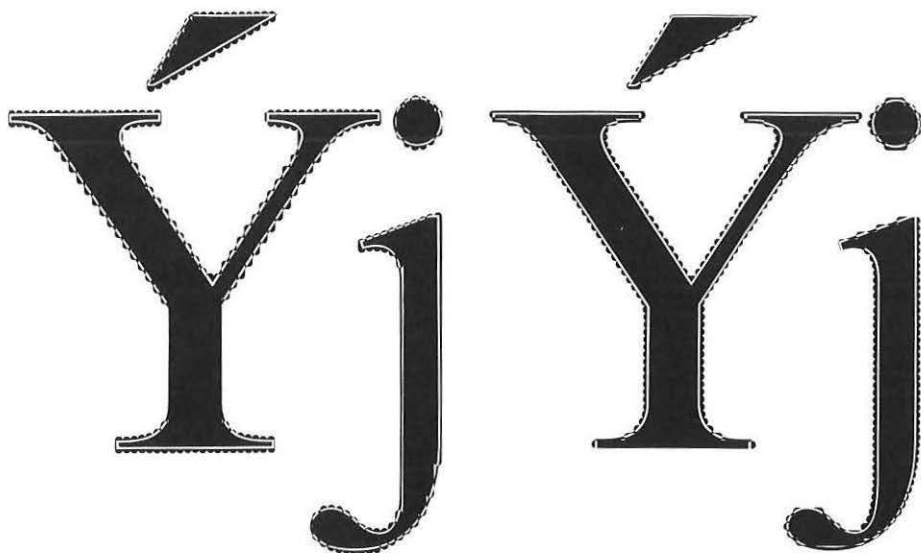
Figure 7. This shows the projected output overlaid with the actual original type forms, to illustrate the growth of the image due to the flying spot tracks where signals are accepted at 50%.
