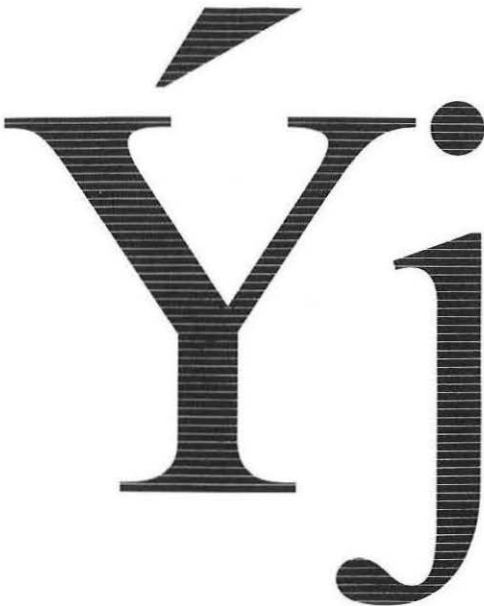
Figure 2. The same characters as Figure 1 broken into 72 horizontal elements with a thickness of 1-1/2% of the body depth. The scan direction is exactly parallel to the width of the characters, and it can be seen how some of the picture elements contain areas where only portions of the element are true image. When such areas are scanned by a flying spot, some decision is necessary to arrange which portions will be acceptable and which will be rejected. An arbitrary decision might be to accept only areas more than 50% true image. If one did this, the scanning system would only register elements in each track where the signal strength exceeds 50%.
