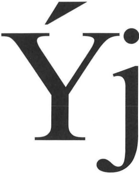
Figure 1. Typical characters in a common type face. The serifs limiting the apparent height of the characters are approximately .003" thick in the 12-point size, which means the ratio of serif thickness to body height is about 50 to 1. One might assume from this that the picture element, or size of flying spot, could not resolve such a narrow area of the image unless it was at least smaller itself. This predicates a flying spot size of substantially less than 1/50'' or 2% of the body depth, just to reproduce in a degenerated way.
