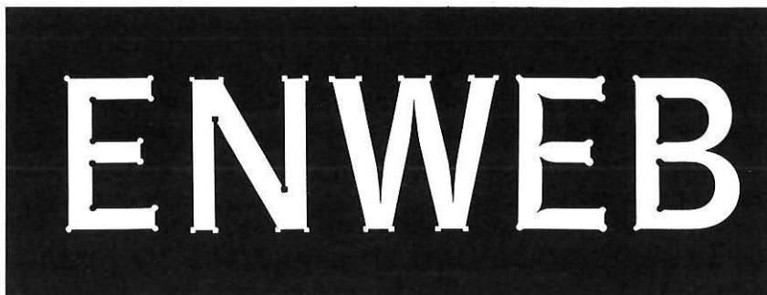
Figure 4. Experimental letters with a variety of differently-shaped lacunae at counter corners and protuberances at outside corner to counteract blooming and decay of televised letterforms.
