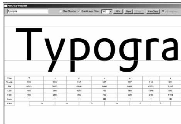
Figure 10 It is possible to check and alter the kerning in the Metrics Editor of both DTL Bezier- and IkarusMaster (from DTL KernMaster screen shot 2007)
